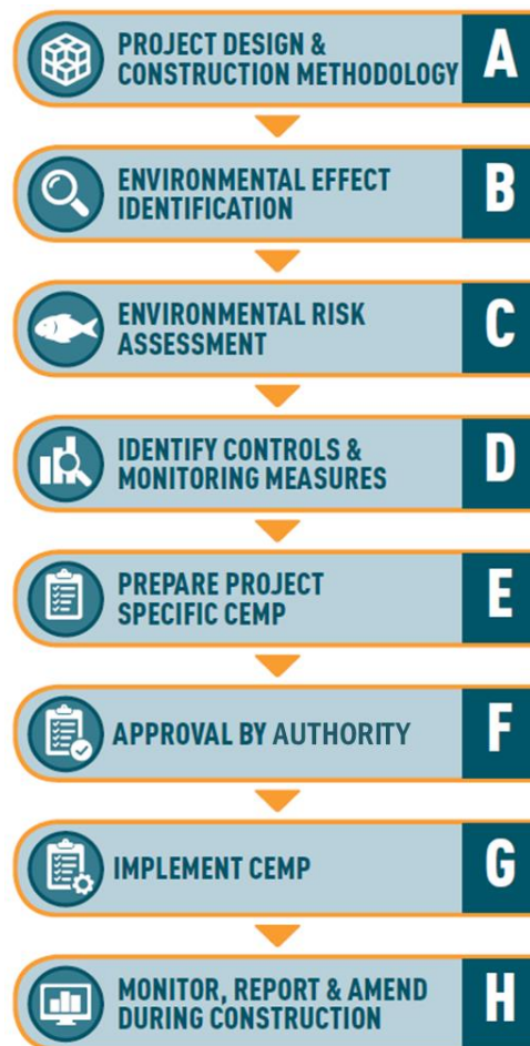
Figure D.1 Process for development and implementation of a construction environmental management plan (source: adapted from LPC 2019)
