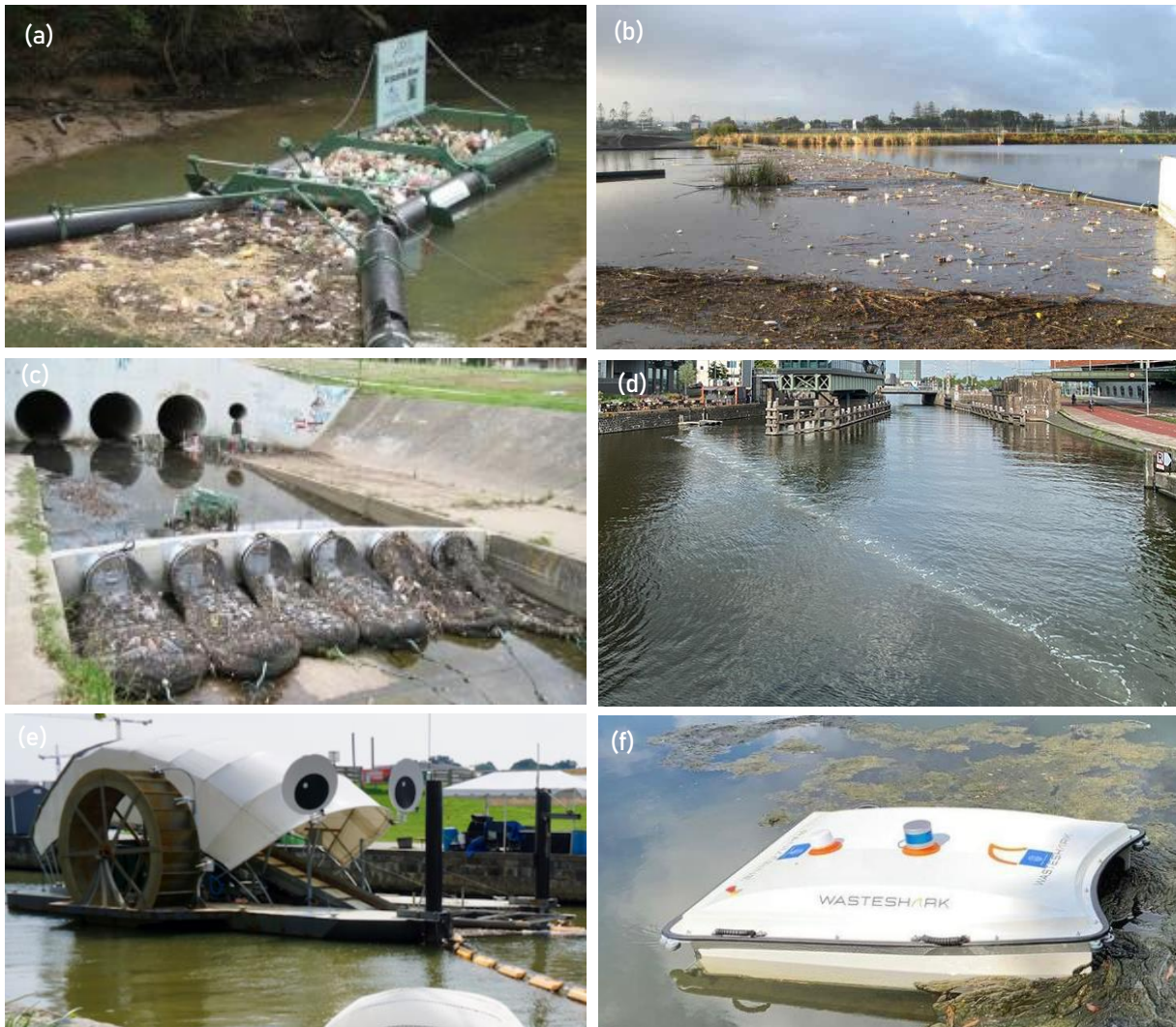
Figure E.15 Examples of a (a) litter trap, (b) litter boom, (c) net trap, (d) barrier (e) litter skimmer and (f) aquatic vacuum (Sources: see Table E.17)
