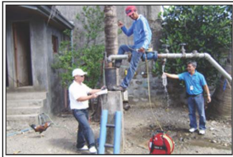
Actual monitoring of groundwater level, water quality and discharge measurement (photo by NWRB staff, 2013)
