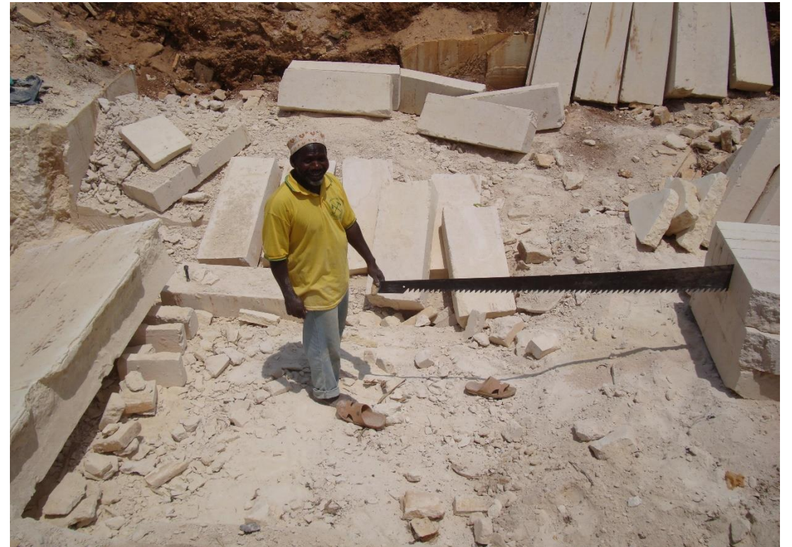
PREPARING LIMETONE BRICKS FOR THE POND SYSTEM
