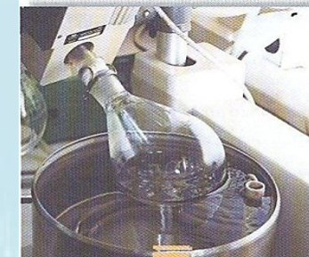
Step 4: The filtrate is evaporated in a Rotavapour
