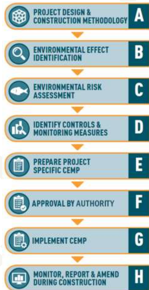
Figure D.3 Process for development and implementation of a construction environmental management plan (source: adapted from LPC 2019)
