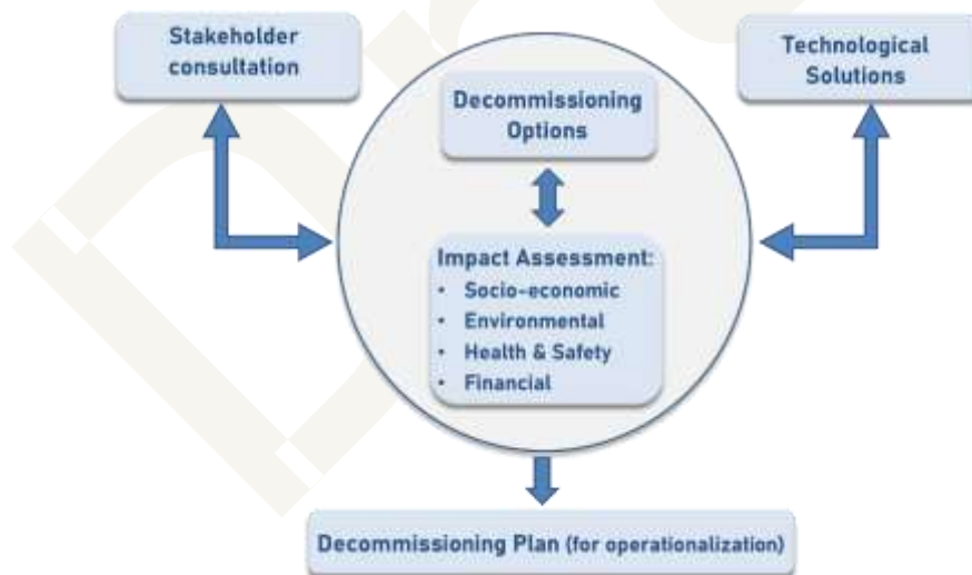
Figure D.4 Conceptual framework for a decommissioning process (adapted da Cunha Jácome Vidal et al. 2022)
